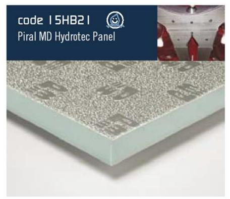
Polyurethane foam panel with  $48 \pm 2$  Kg/m³ density, 20 mm thickness, coated on both sides with 60-micron thick aluminium foil. This coating is protected on one side with 2 g/m² antioxidant lacquer based on polyester and on the other by thermo-welding lacquer based on vinyl resin. This panel is especially suited for use in air-conditioning and heating system installations.  $48 \text{ m}^2$  pack.
