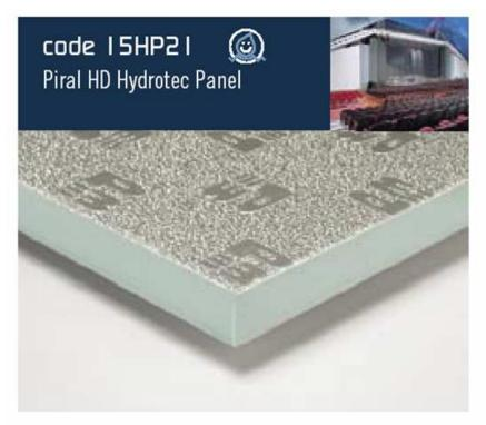
Polyurethane foam panel with  $52 \pm 2$  Kg/m³ density, 20 mm thickness, coated on both sides with 80-micron thick aluminium foil. The aluminium foil is embossed on both sides and coupled with a 2 g/m² layer of corrosion-resistant polyester paint. This panel is especially suited for use in air-conditioning and heating system installations.
